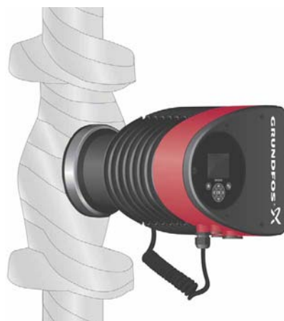
Fig. 15 Insulation of pump housing and pipework
